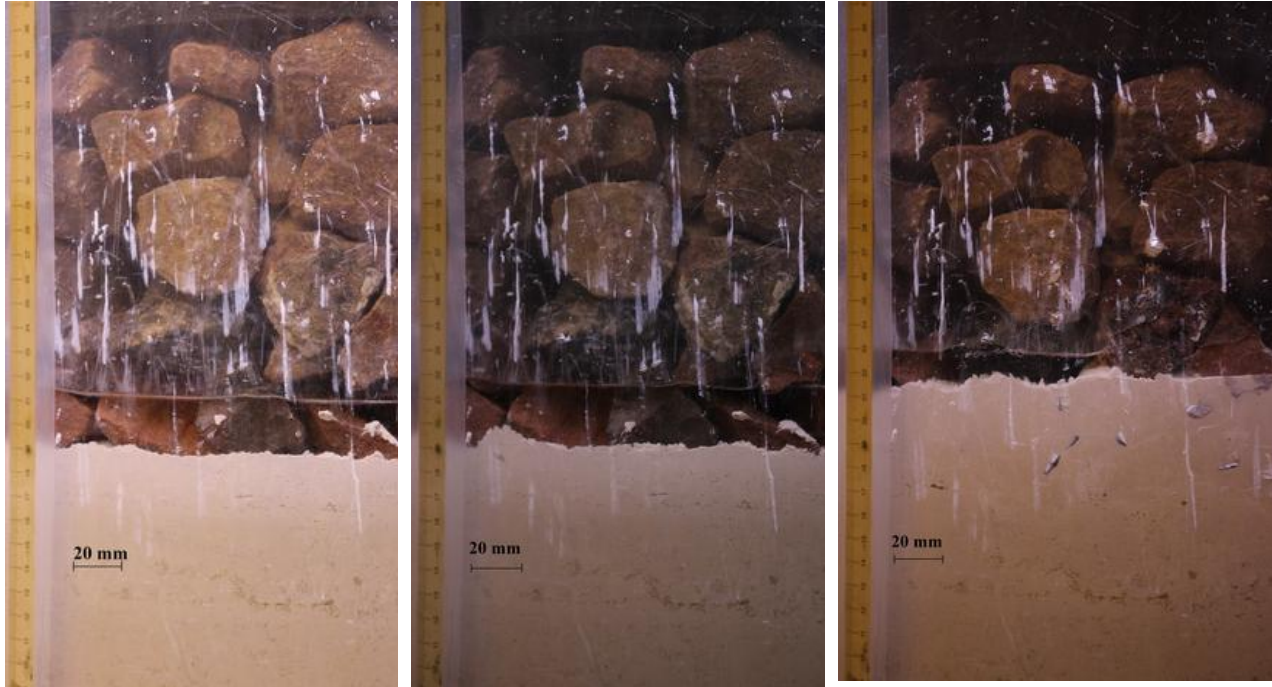
a) After saturation and before monotonic loading b) After monotonic loading (saturated state) c) After cyclic loading (saturated state)
